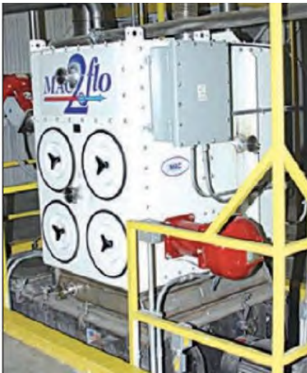
Baghouses feature cartridge filtration, explosion suppression, and clean-in-place design
