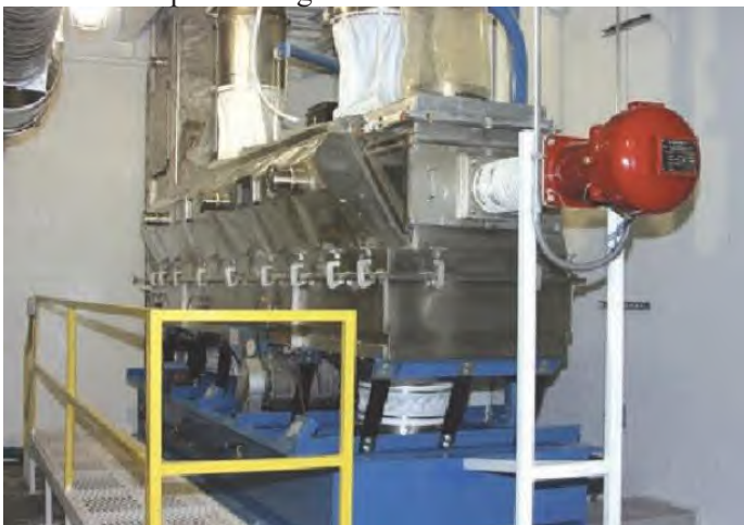
We utilize vibrating fluid bed dryers to ensure correct moisture levels in finished product
