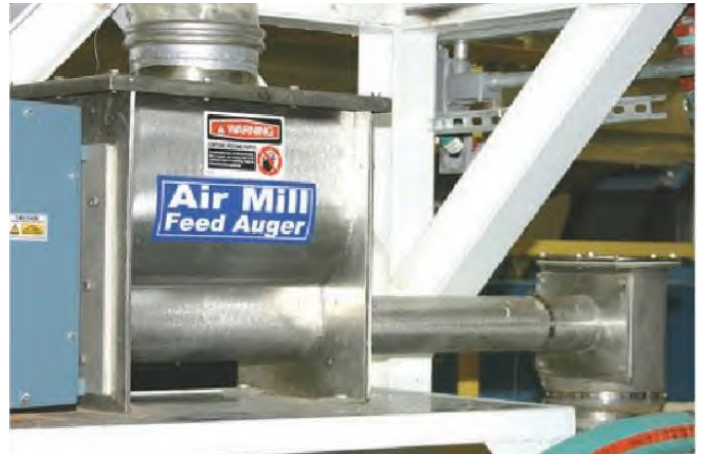
Stainless steel augers promote years of corrosion-free operation
